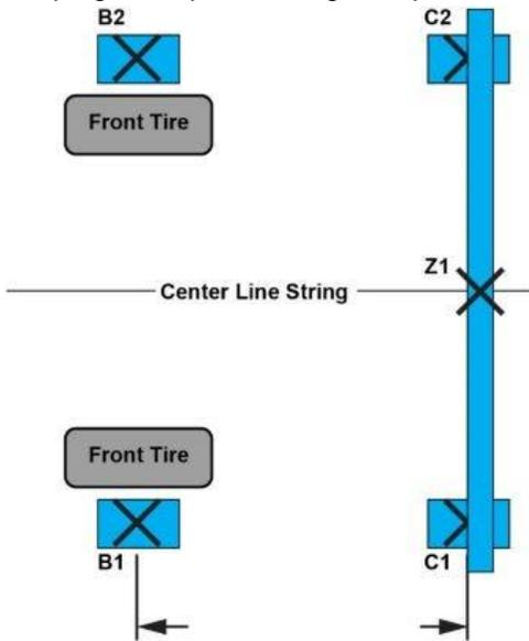
13. Make a new mark where the center line string intersects the tape edge. We will call this mark Z1. This mark should be bold and very visible as you will place the target stand on it later.
