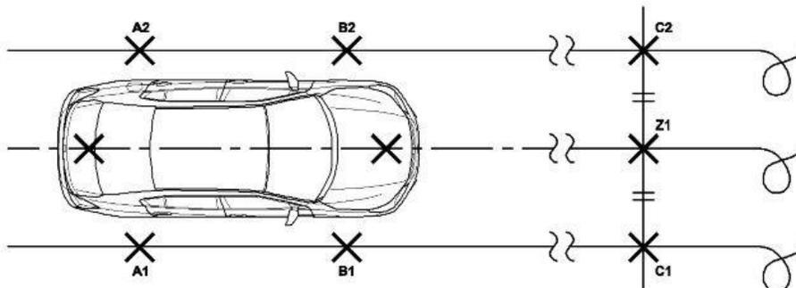
Some models, like the Accord and Civic, will require an additional reference mark as the radar is mounted to the side. This mark can be simply made on the tape placed in step 12. Refer to the aiming procedure for additional information.
