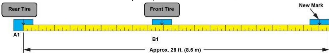
10. Move the start of the tape measure to B1 while aligned with C1, and make a new mark according to the distance listed in the service information procedure.
