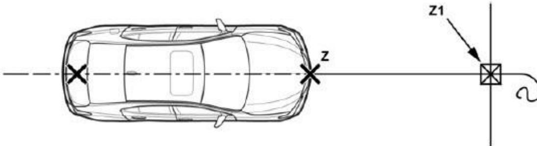
1. Determine the centerline at the rear of the vehicle, and position the gas shock with the cord or string attached. Refer to the procedure Before Aiming Setting in the service information.
