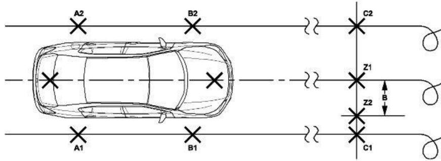
The procedure mentioned can also be used when setting up the LaneWatch camera aiming. Instead of in front of the vehicle, use the procedure to set up the reference marks behind the vehicle.
