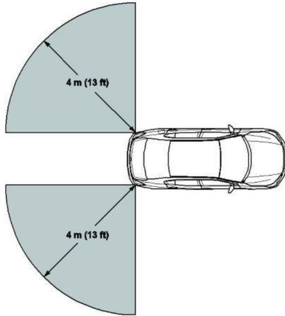
**Radar, FCW/LDW Camera, or Multipurpose Camera Aiming**
