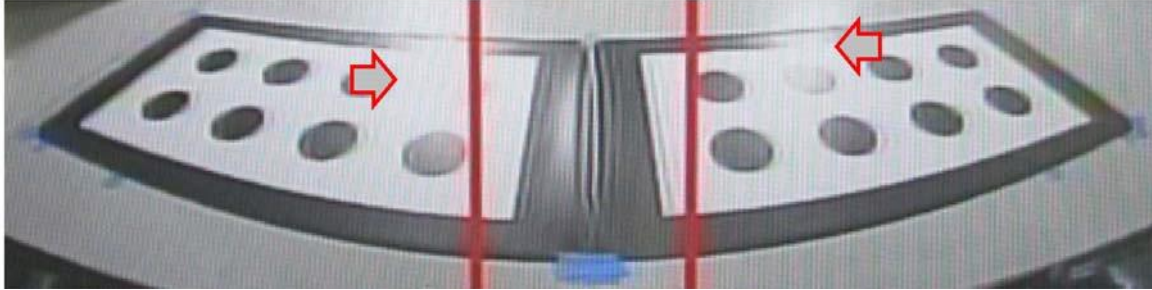
Reflection or glare on the target dots
